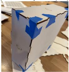
Once this is done, ensure you've added enough supporting tape to the joins so they stay well connected while the wood glue dries.
