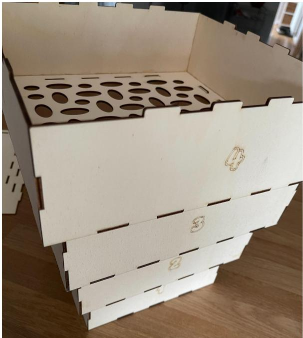
You can now load the top level with Bricks (don't over fill) and shake the column of boxes so that the smaller items move to the lower tray. If you want you can use the lid to stop bricks from falling out a top level when shaking.
