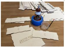
Place glue at the bottom of a side panel, where that panel and the bottom plate will connect. I've found it easiest to place glue using a small brush helps reduce any spreading glue. Push them together.
