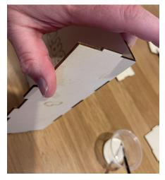
Then place tape on the joins to keep the pieces connected
